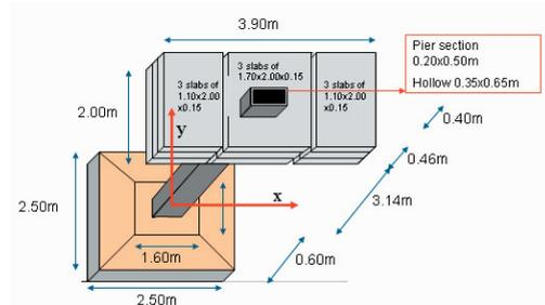
Figure 2. Geometry of the model bridge pier
