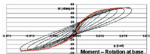
Figure 8. Observed cyclic behavior of pier A2 tested at the strong reaction frame (Moment – Rotation).
