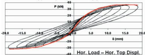
Figure 7. Observed cyclic behavior of pier A2 tested at the strong reaction frame (Horizontal Load – Horizontal Displacement  $H = 1.42\text{m}$ ).
