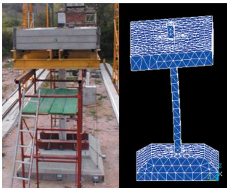
Figure 12. 3D FE model and 1<sup>st</sup> natural period with the use of the commercial FE package ANSYS
