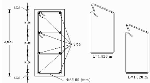
Figure 5. Dimensions and reinforcing details of Volvi pier cross-section (Models A1, A2 and B1)
