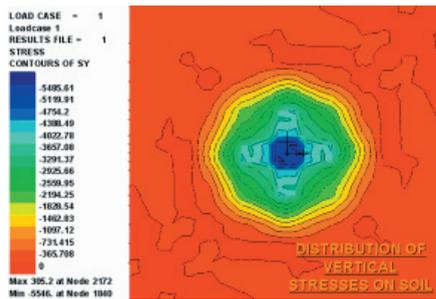
Figure 10. Distribution of expected vertical stresses on soil
