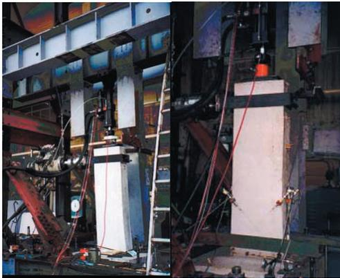
Figure 3. Pier A1 or A2 subjected to cyclic testing
