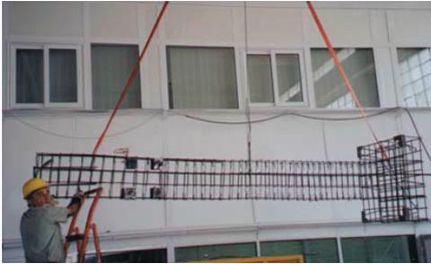
Figure 6. Dimensions and reinforcing details of Volvi pier cross-section (Models A1 and A2)
