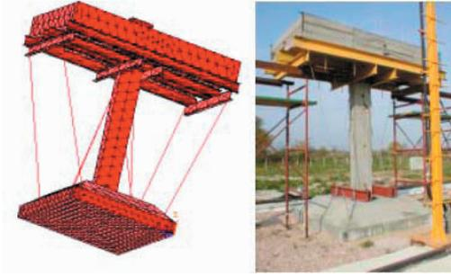
Figure 9. Complete FE model inclusive of the additional steel section for the pier-deck connection and the restraint cables for the foundation-deck connection.
