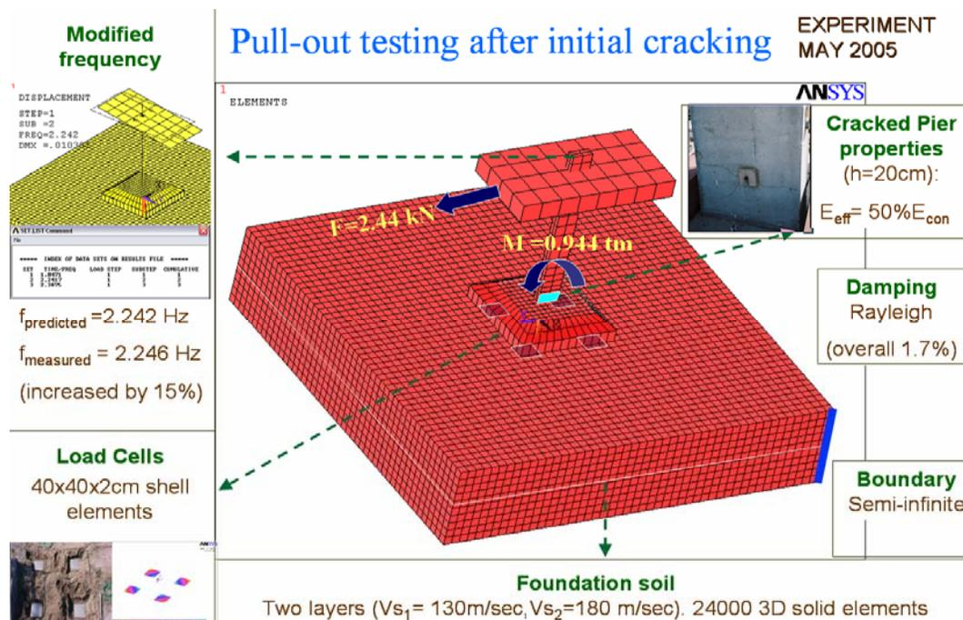
Figure 13: Overview of the FE model for the case of the post-cracking pull-out tests
