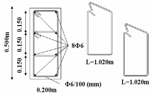
Figure 4. Basic cross-section of the pier model
