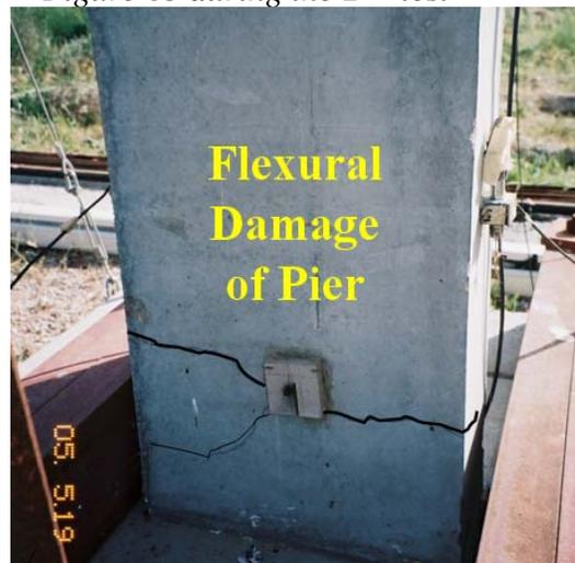
*Figure 7: Flexural damage of the pier near its base after the 19th May 2005 experiment (cracking has been accentuated in this figure to become visible)*
