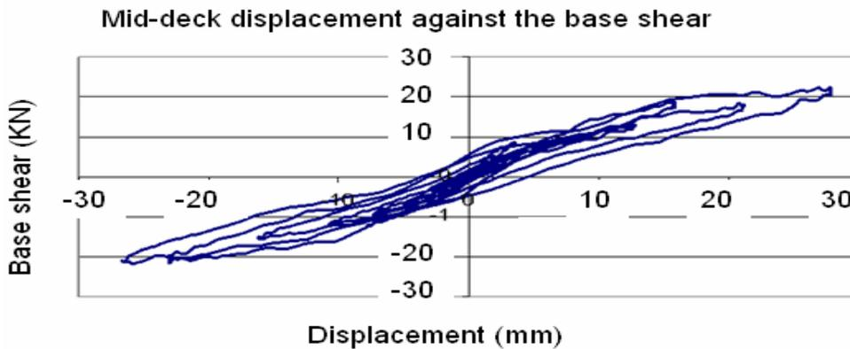
Figure 8: Base shear force - displacement response at the middle of the Deck 2<sup>nd</sup> low-to-medium intensity test, 19<sup>th</sup> May 2005). Model with cables and struts
