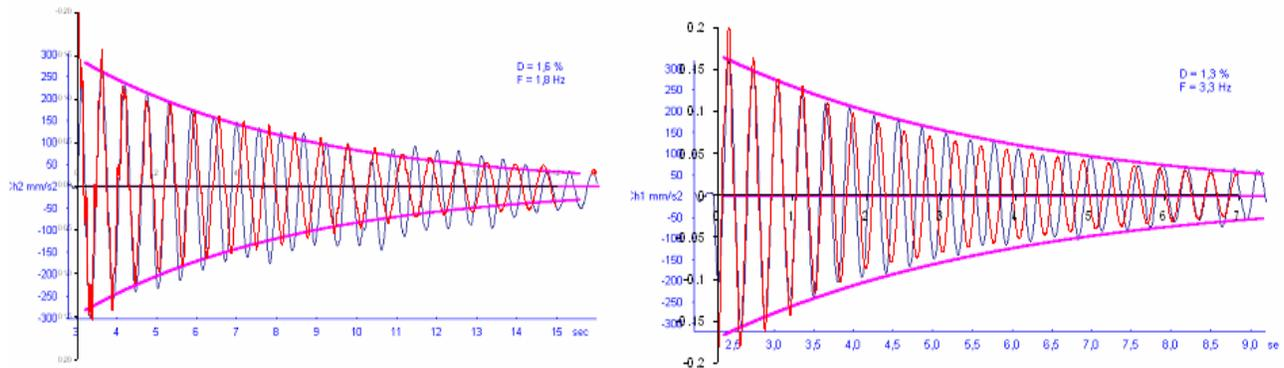
Figure 9: Low-intensity pull-out test 13<sup>th</sup> May 2004. Left: Deck horizontal acceleration response. Out-of-plane direction. Right: Deck horizontal acceleration response. In-plane direction (Numerical predictions in red color).
