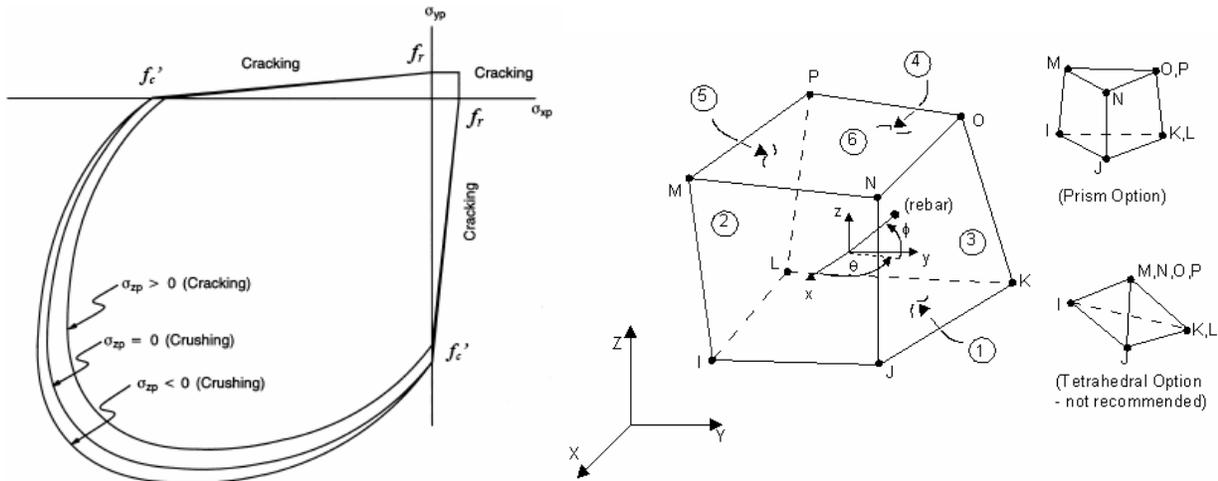
Figure 11: Failure criterion implemented into the SOLID65 special concrete element of ANSYS
