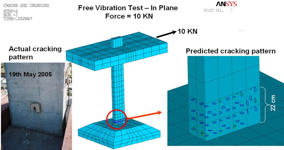
Figure 12: Numerical prediction of the pier non-linear response using the cracking and crushing capabilities of ANSYS for concrete
