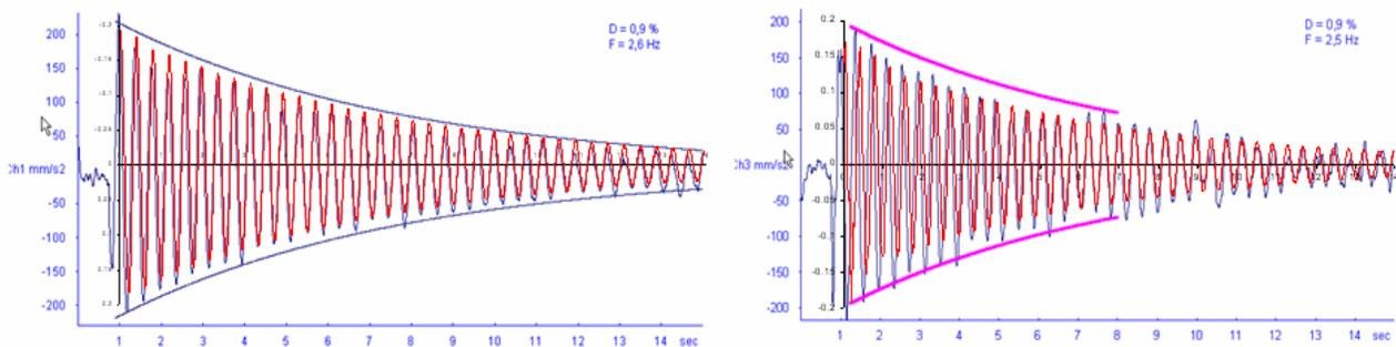
Figure 10: Low-intensity pull-out test 20<sup>th</sup> October 2004. Left: Deck horizontal acceleration response. In-plane direction. Right: Deck vertical acceleration response. (Numerical predictions in red color).
