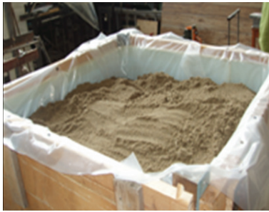
Figure 6a. 1 st Shear stack with wooden sections.
