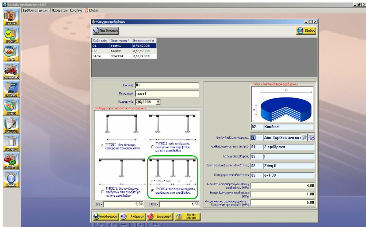
Figure 8. Overview of the software developed for the preliminary selection of the overpass bearings.
