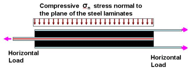
Figure 1b. Slice bearing specimen
