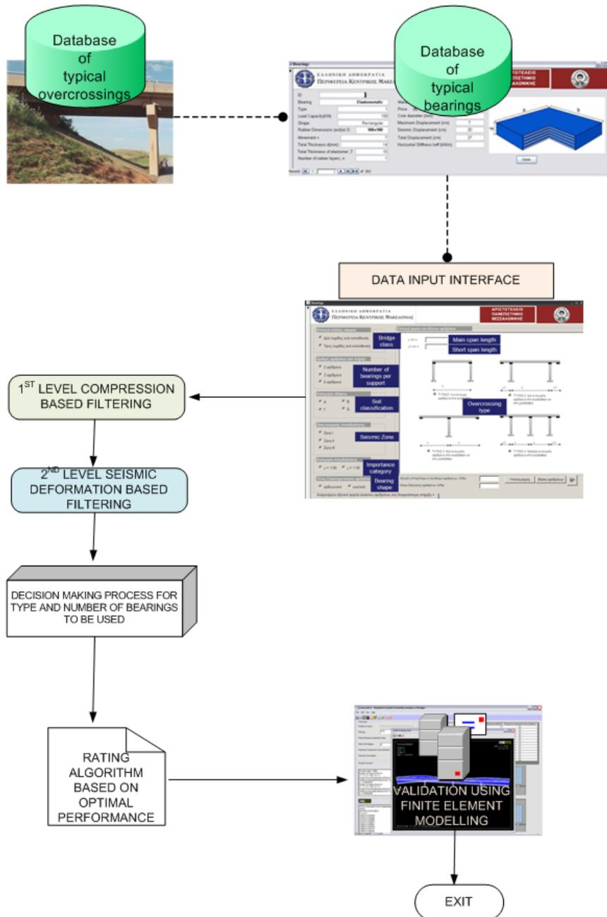
Figure 7. Overview of the software structure
