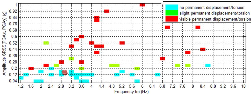
Figure 6. Rocking spectra for the Roman Colonnade under seismic-hazard compatible ground motion scenarios. Thessaloniki (1978) earthquake strong ground motion record depicted as a circle.
