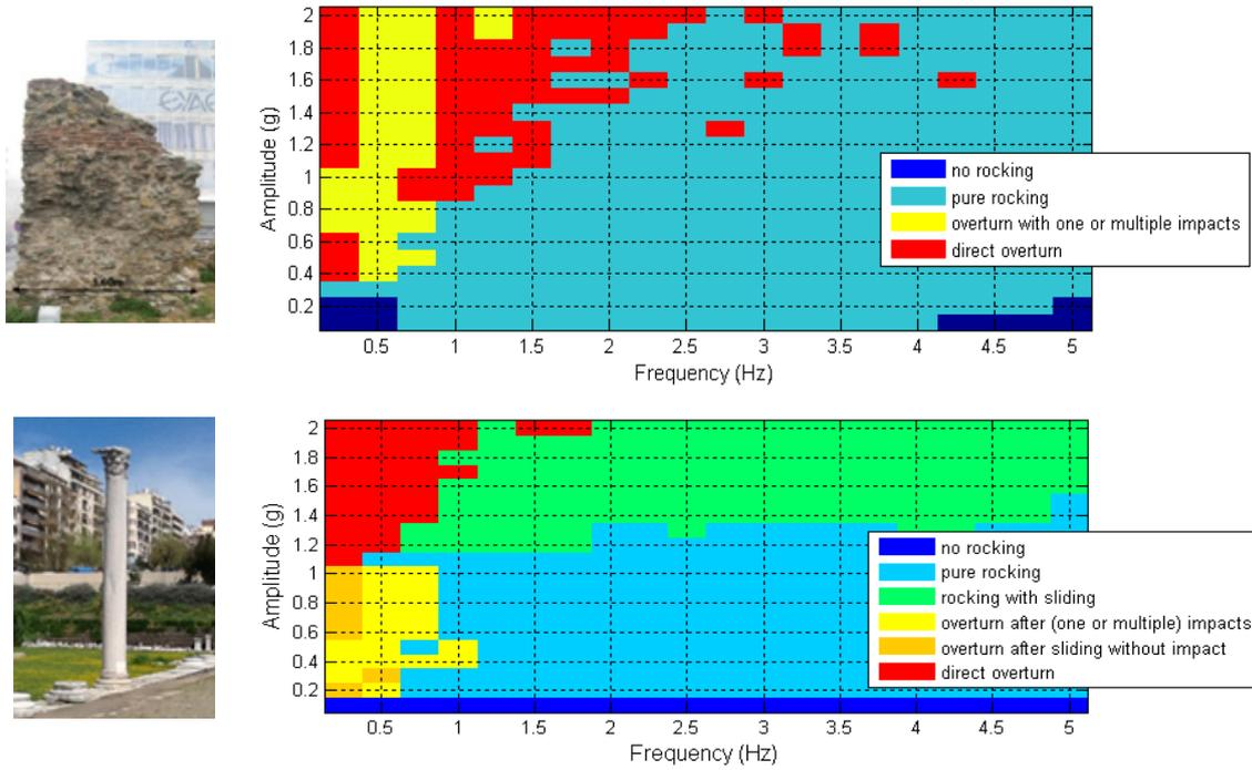
Figure 5. Rocking spectra for the two systems under harmonic excitation  $f(t)=\cos(\omega t)$ .
