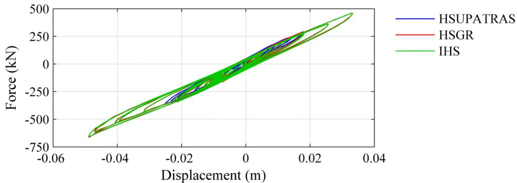
Figure 4. Comparison of the force–displacement loops for the three experiments.
