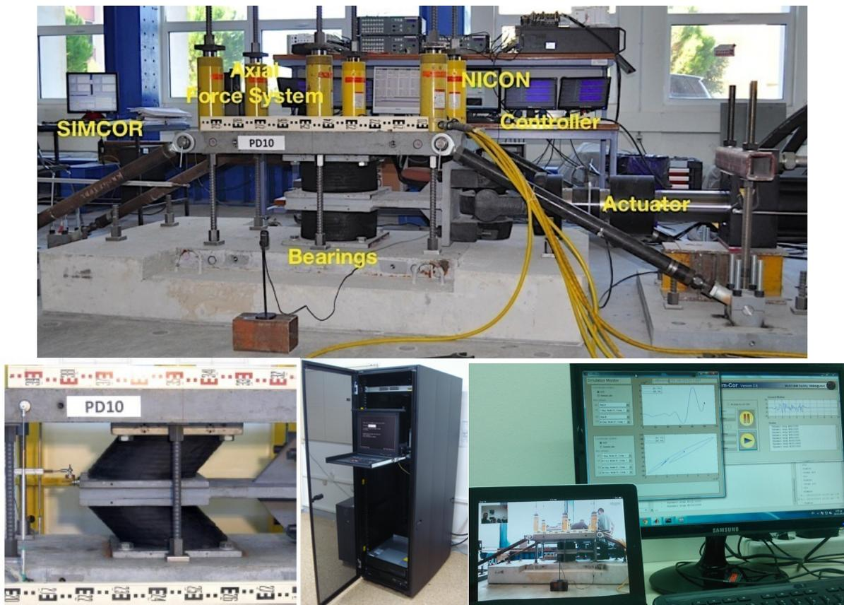
Figure 3. Experimental setup (top) and bearings tested (bottom, left) at the University of Patras along with the computational server at the University of Thessaloniki (bottom, right)
