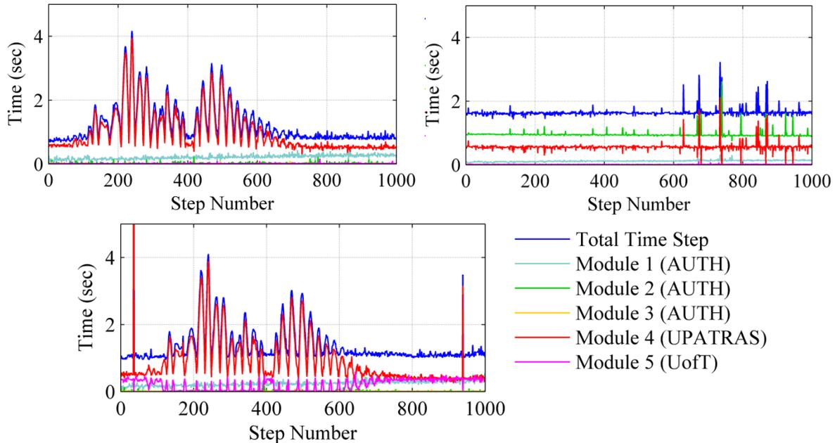
Figure 5. Time step delay for the intercontinental multi-platform simulation (IMPS, top left) hybrid simulation between Greek partners (HSGR, top right) and the intercontinental hybrid experiment (IHS, bottom).
