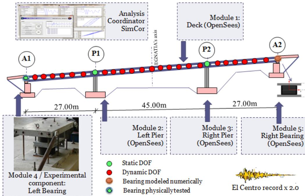
Figure 2. Layout of the bridge substructuring for the multi-platform and the hybrid simulation.
