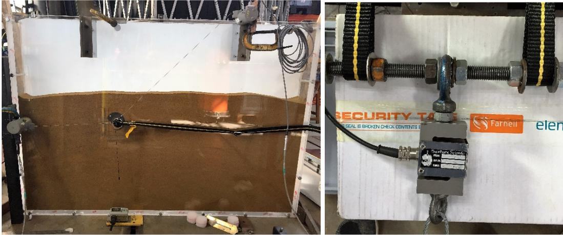
Figure 3: Photographs of experimental setup, during filling of a preliminary loose experiment (left) the load transfer mechanism with load cell (right).
