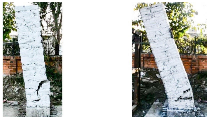
Figure 11 Final deflected shape of the unretrofitted (left) and retrofitted (right) wall before collapse
