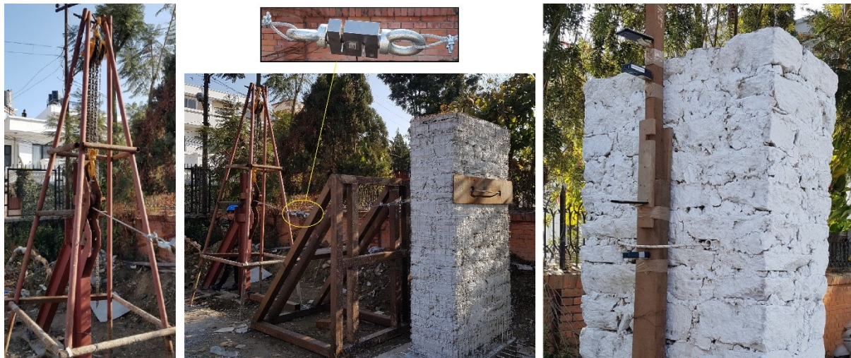
Figure 9 Chain pulley arrangement (left); Pulldown setup for retrofitted wall (mid); Lasers placed pointing towards the retrofitted wall, using the unretrofitted wall as support (right)
