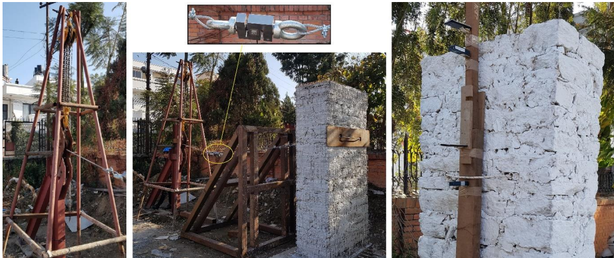
Figure 5 Chain pulley arrangement (left); Pull-down setup for retrofitted wall (mid); Lasers placed pointing towards the retrofitted wall, using the non-retrofitted wall as support (right)
