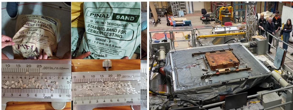
Figure 1.2 Alternative sand samples tested (left) and PVC-s moderate scale testing campaign on the shaking table of the University of Bristol (right).
